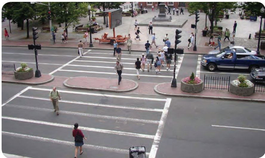
Medians and clearly marked crossings increase safety and direct pedestrian flow.
