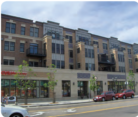
Architectural massing avoids overwhelming the pedestrian realm by stepping back as the building height increases.
